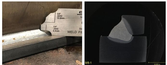
Figure 5. TW-GMAW weld made at a total wire feed input rate of 940 ipm with a travel speed of 25 ipm: weld visual appearance (left) and metallographic cross-section (right).
